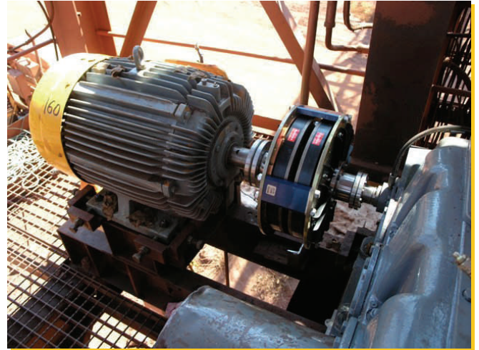
▲ MGD 18/250, 150HP, 1500RPM, Iron Mill, Australia
