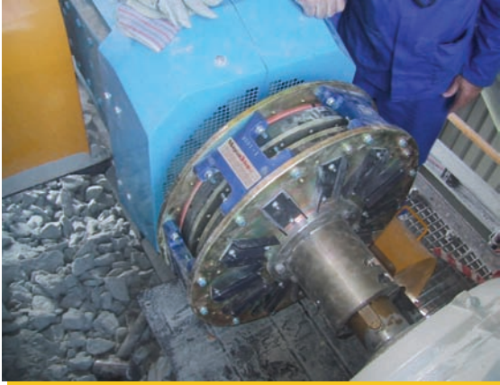
▲ MGD 20/400, 250HP, 1500 RPM, Conveyor System, Mining, Botswana
