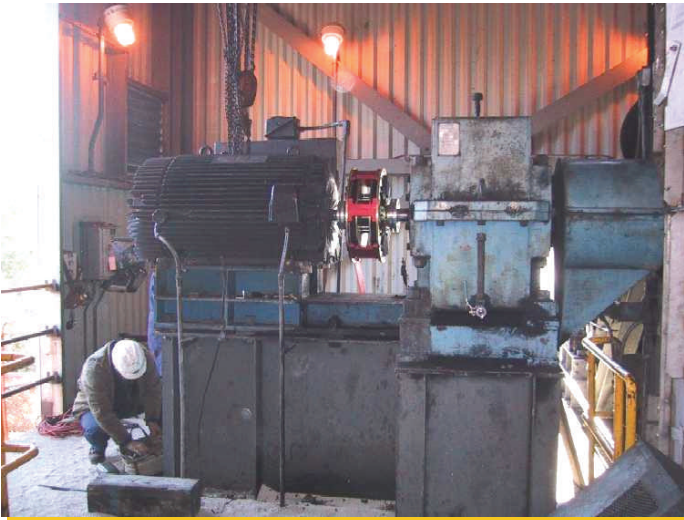
▲ MGTL 18/250, 240HP, 1800RPM, Mining, Conveyor System, UT, USA
